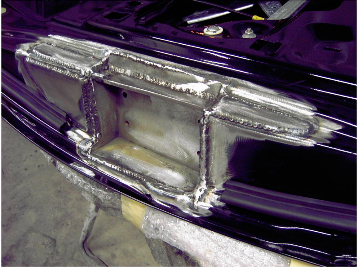
7. Test the motion of the door to take care of any interferences and alignment issues. Use shims or washers between the hinge and the boxes for fine tuning but make sure you have enough threads left to hold the hinge properly. You can also ovalize the box holes to achieve desired alignment.
